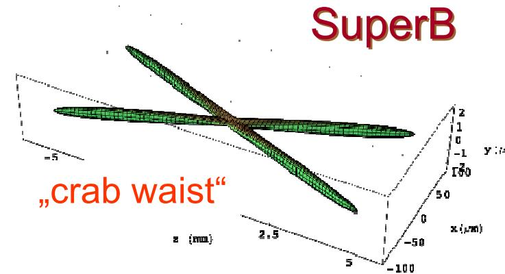
Main gain in lumi from bunch size:  $\sigma_y = 35 \text{ nm}$ ,  $\sigma_x = 5 \mu\text{m}$ ,  $\sigma_z = 6 \text{ mm}$ ,
